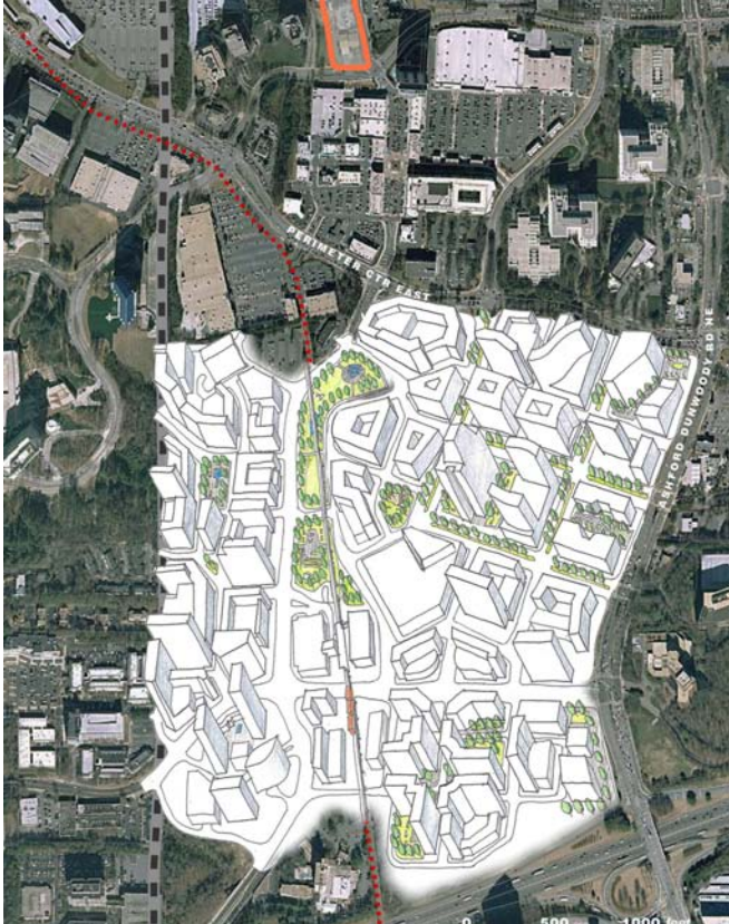
Phase Four - Mall retrofit - Establishing street grid and block structure with civic spaces - 3D illustration
